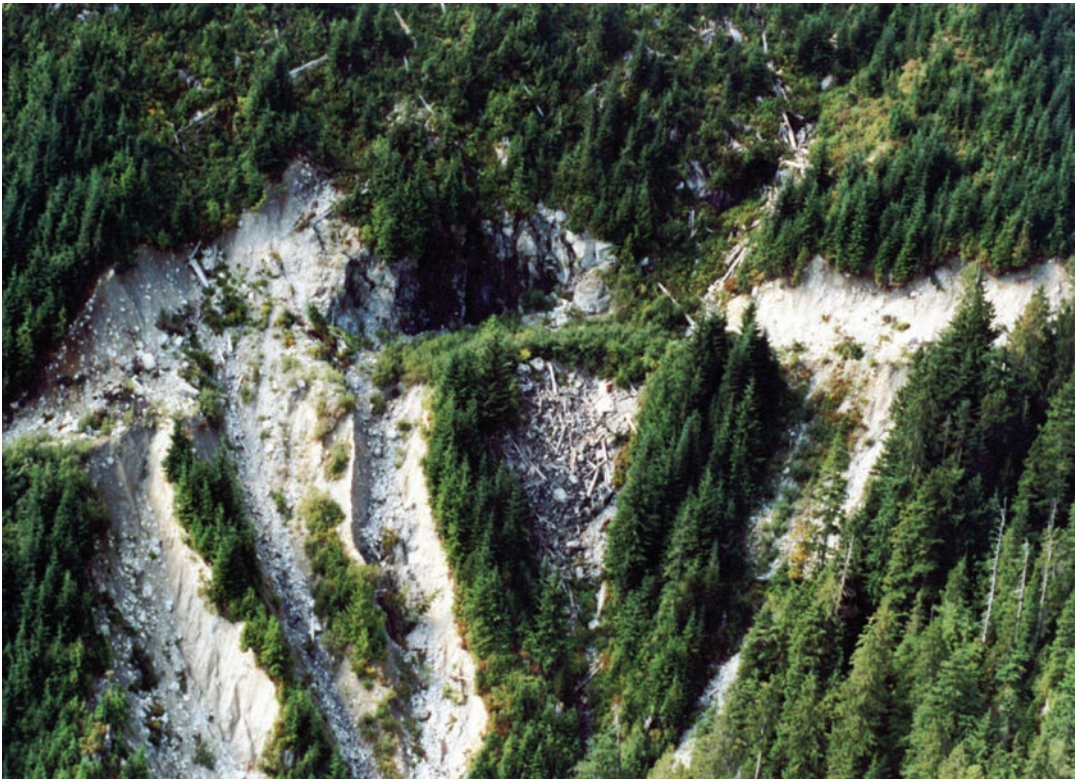
Landslide associated with a logging road and clearcuts
